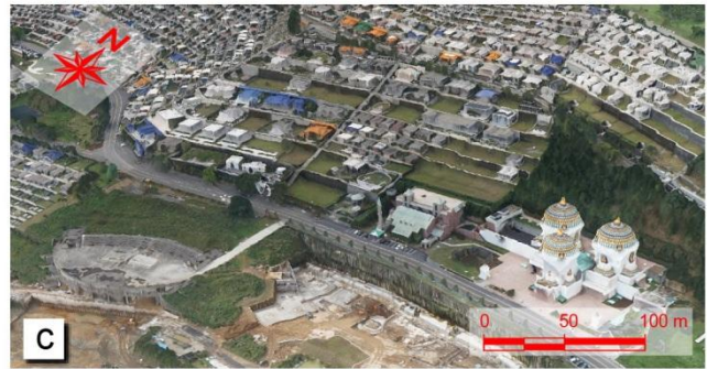
Fig. 2: Data acquisition from an unmanned aircraft system flight mission. (a) DSM generated by the UAS for a total area of 14.7 km 2 with a GSD of 6.6 cm, where points and lines represent the positions and path of the flight mission, respectively, and the monotone gray area is the LiDAR DSM; (b) side view of the hillshaded true 3D model; and (c) image draped onto the true 3D model. The side views of (b) and (c) are captured at the same position and orientation.
