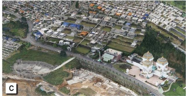
5 **Figure 3: Data acquisition from an unmanned aircraft system flight mission. (a) DSM generated by the UAS for a total area of 14.7 km<sup>2</sup> with a GSD of 6.6 cm, where points and lines represent the positions and path of the flight mission, respectively, and the monotone gray area is the LiDAR DSM; (b) side view of the hillshaded true 3D model; and (c) image draped onto the true 3D model. The side views of (b) and (c) are captured at the same position and orientation.**
