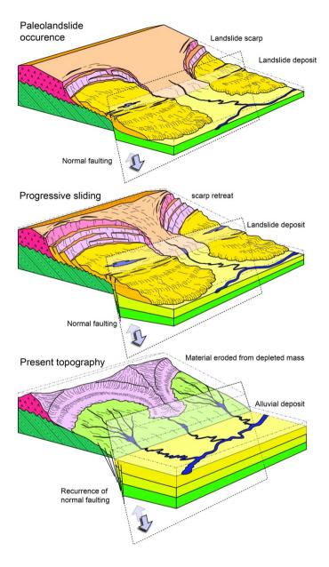
Figure 14: Schematic illustration of the evolution of the landslides. The triggering mechanism may be associated with normal faulting of the JSF (also known as the SCF), which transects the slope toe. The accumulation zone crossing the fault was eroded and transported, resulting in the current plain, as shown in the lower figure.
