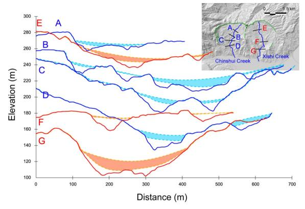
Figure 12: Cross-sections of the river valleys situated in the landslide area. The shaded area indicates the possible datum ranges obtained within various search radii (D1 and D2 in Fig. 10b). If the current elevation is lower than the possible paleodatum, this depth represents the amount of the incision. The upper and lower bounds are indicated by the semiopaque dashed line. The locations of the cross-sections in the landslide area are shown in the inset.
