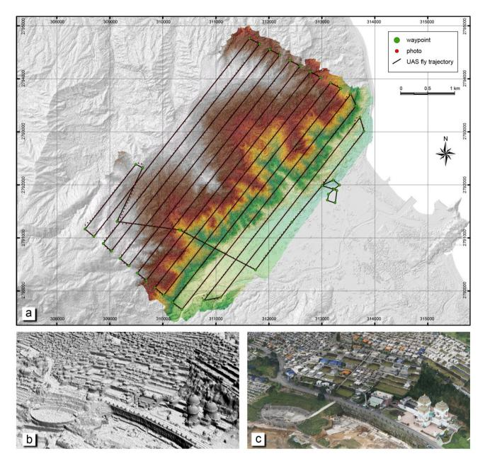
Figure 3: Data acquisition from an unmanned aircraft system flight mission. (a) DSM generated by the UAS for a total area of  $14.7~\rm km^2$  with a GSD of  $6.6~\rm cm$ , where points and lines represent the positions and path of the flight mission, respectively, and the monotone gray area is the LiDAR DSM; (b) side view of the hillshaded true 3D model; and (c) image draped onto the true 3D model. The side views of (b) and (c) are captured at the same position and orientation.
