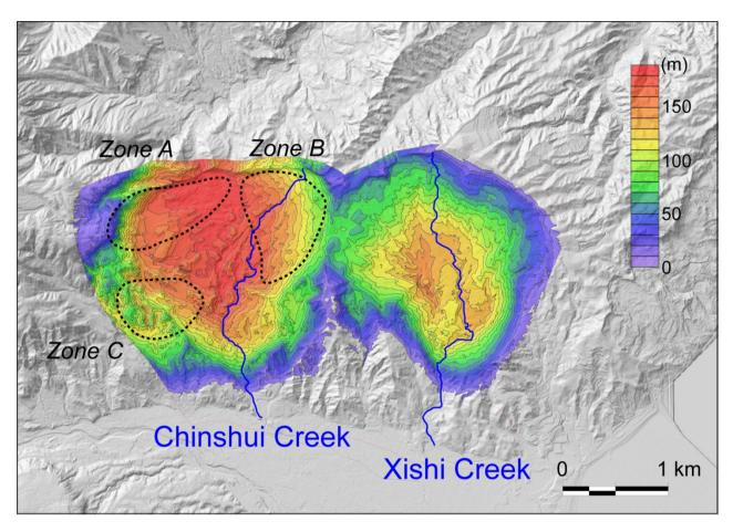
Figure 11: Isopach map of the landslides. The depleted landslide mass is calculated from the difference in height between the current and reconstructed topographies. The contour bands are shown at 10-m intervals.
