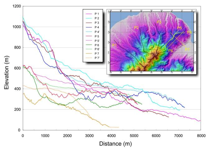
Figure 9: Topographic profiles of the Tatun volcanic cone. For P4, P5, and P6, profiles from the original (solid line) and the reconstructed (dashed line) DEMs are shown. The profile locations are shown in the inset in the upper right corner.
