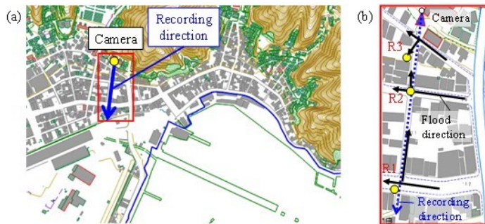
Figure 12: Location of video recording: (a) shooting direction and (b) crossings for measurement.
