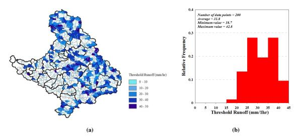
Figure 5: (a) Threshold runoff and (b) the relative frequency of runoff.
