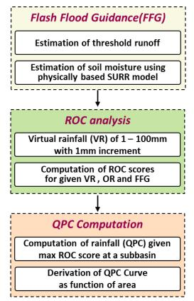
Figure 1: Overall methodology used to estimate the quantitative precipitation criteria.
