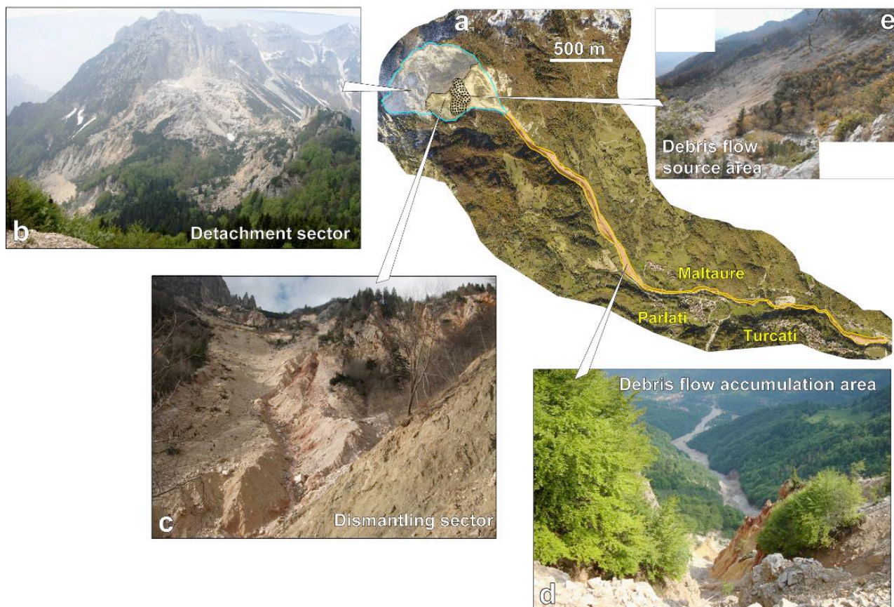
167 168 Figure 2. The Mt. Rotolon DSGSD plan (a); landslide sectors (b, c) and the 2010 debris flow features (d, e).
