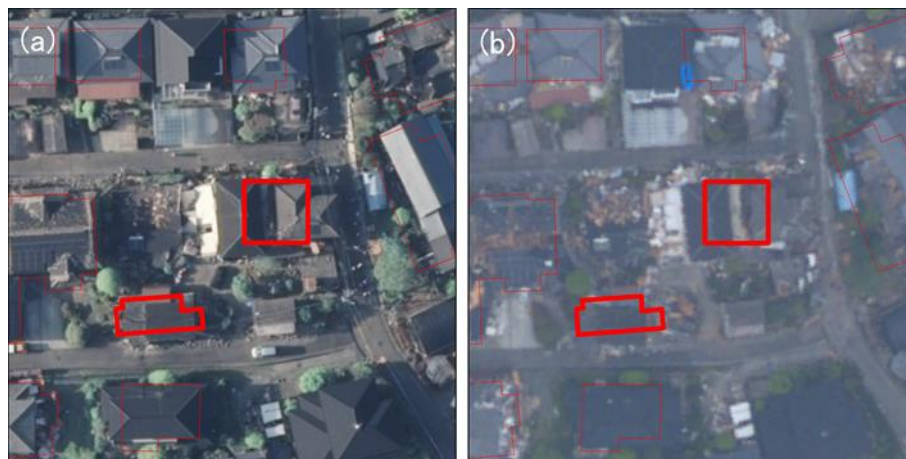
Figure 15: (a) Aerial image taken on April 15; (b) Aerial image taken on April 23. The thick red polygons shows buildings that collapsed after the foreshock and were detected using the \Delta H threshold.
