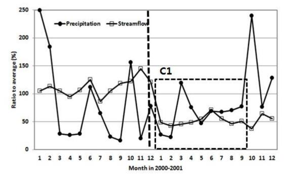
(d) Monthly time series of monthly precipitation and streamflow at sub-basin 3014 in 2000-2001
