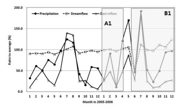
(b) Monthly time series of precipitation, streamflow, and dam inflow at sub-basin 3001 in 2005-2006
