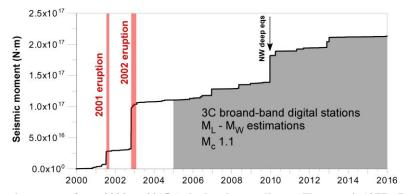
Figure 3: Cumulative seismic moment from 2000 to 2015 (calculated according to Kanamori, 1977). The periods marked in red indicate the main flank eruptions; in grey the time-span selected for the analysis. Note that the step in the seismic release at the end of 2009 is related with a seismic sequence occurred in the NW sector of Etna at a depth of 24-28 km, not affecting the characterization of shallow seismicity.
