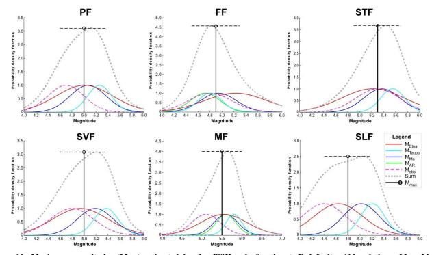
Figure 11: Maximum magnitudes ( $M_{max}$ ) estimated by the FiSH code for the studied faults. Abbreviations:  $M_{Etna}$ - $M_{Taupo}$ , magnitude from earthquake scaling relationships for Etna and Taupo;  $M_{Mo}$ , scalar seismic moment magnitude;  $M_{AR}$ , magnitude from aspect ratio relationships;  $M_{obs}$ , maximum observed magnitude. Uncertainties are represented by probability curves (see text for explanation).
