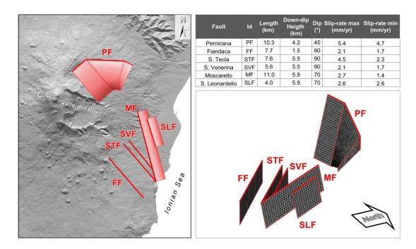
Figure 9: Pattern of individual sources used in the geological model and related geometric-kinematic parameters: red boxes in the left frame represent the projection at the surface of the fault planes, lines indicate the vertical planes. Note that lengths refer to the seismogenic fault segments only, whereas the ones governed by prevailingly creeping behaviour are not considered.
