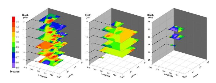
Figure 8: Distribution of the b-values beneath Etna calculated from the instrumental earthquake catalogue (2005-2015): the horizontal sections show the grids at different depths.
