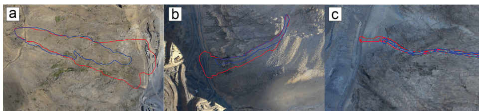
Fig. 15. Comparison between avalanche run out distance using cold ( T_0 = -10^\circ\text{C} , blue line) and warm snow ( T_0 = 0^\circ\text{C} , red line) for the (a) LGW-2 , (b) BN-1 and (c) CCHN-3 case studies. Warm snow leads to more frictional melting and longer avalanche runout.
