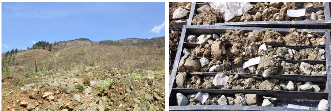
253 254 (a) Material on the landslide surface (b) Material in the shear zone
