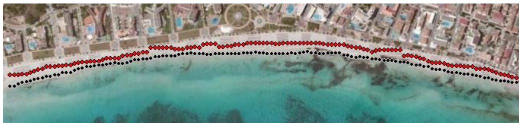
Figure 15: Present-day shoreline position in (black) and landward migration (in red) in the worst case scenario (mean sea level rise under RCP85 and extreme wave conditions) by the end of the 21st century in Cala Millor beach.
