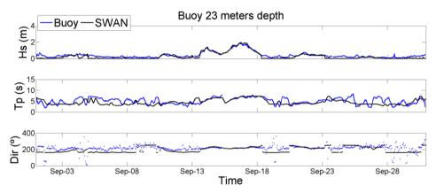
5 Figure 910: Hs, Tp and wave direction as modelled by SWAN model and observed at the buoy deployed at 23 m depth in Playa de Palma beach.
