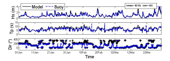
Figure 65 Capdepera buoy observations (blue) and hindcasted SIMAR (black) time series of Hs, Tp and wave direction. RMSE and correlation are quoted for the wave direction (for Hs and Tp the values are quoted in Figure 6).
