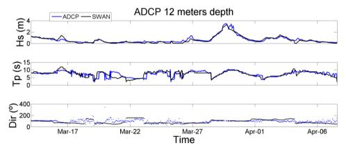
Figure <u>8</u>7: Hs, Tp and wave direction as modelled by SWAN and observed at the ADCP deployed at 12m depth in Cala Millor beach.
