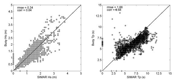
Figure 7:6 Scatter plots of buoy observations vs SIMAR hindcast for Hs (left) and Tp (right). RMSE and correlation are quoted in each figure.
