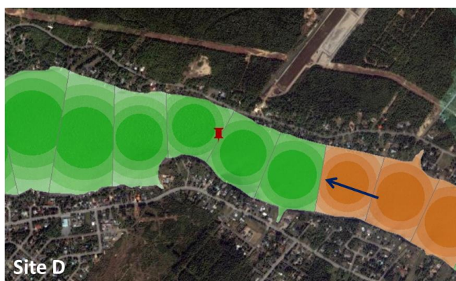
290 Figure 10: False-negative error on the St-François River with no apparent explanation. The arrow indicates flow direction.
