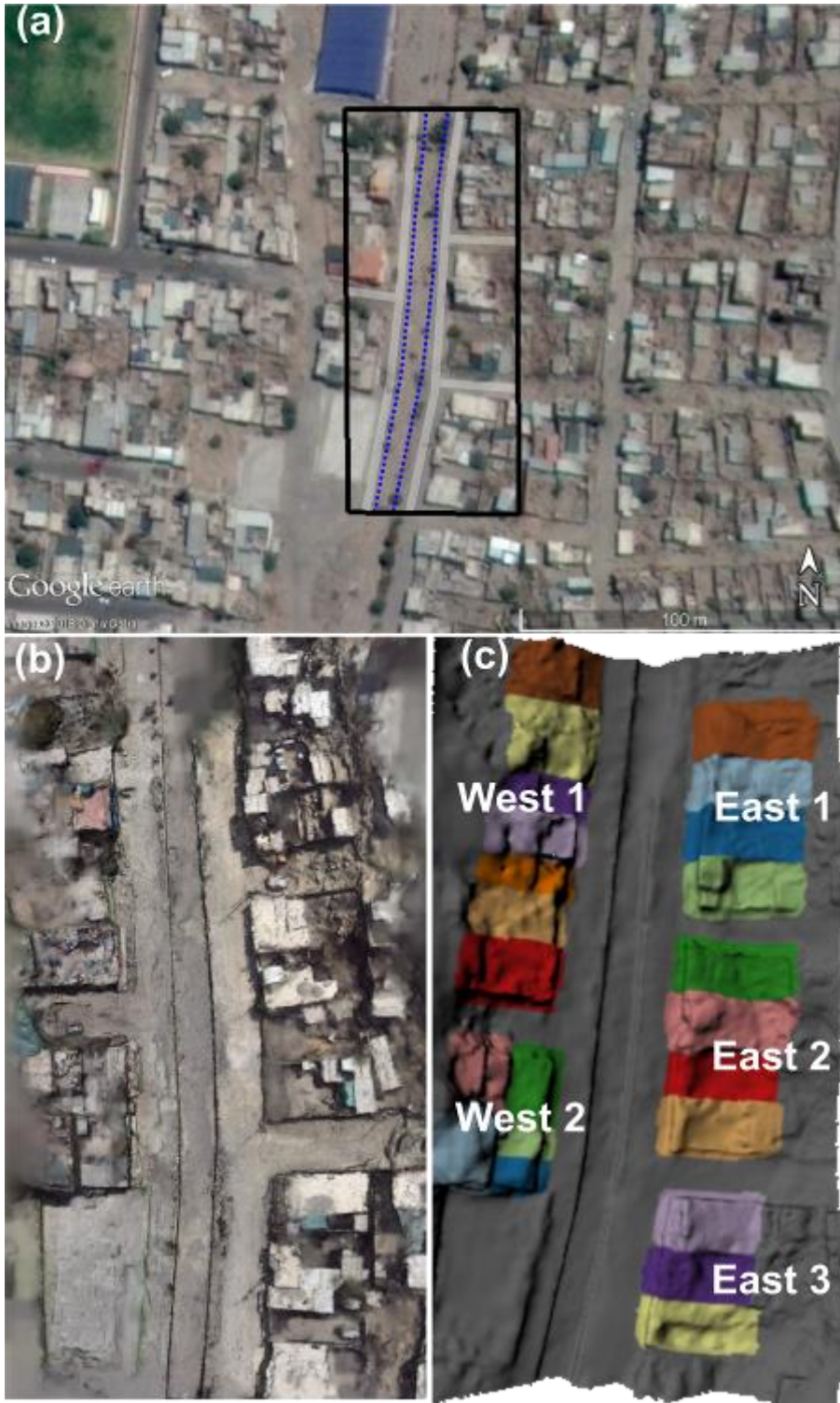
Figure 2. Overview of Quebrada Dahlia study area, Arequipa, (a) aerial image with black outline showing study area, dashed outline showing channel banks and transparent lines showing streets in the area, (b) photogrammetric reconstruction of the surface and (c) individual buildings and building blocks identified from building surveys.
