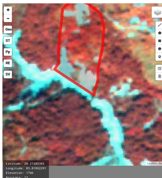
Figure 6 : Offline Component with a satellite image as a background: Geolocation (Geo), Stop Geolocation (ST), Show all the attributes in a pop up window (Pp), Reset the map (RE) Save as Geojson-TXT (SV)
