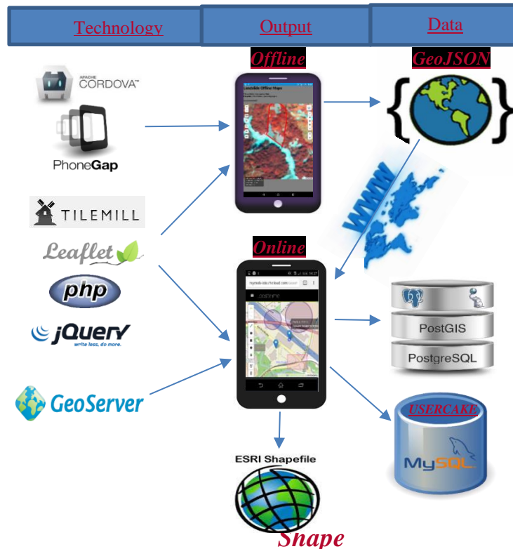
Figure 5: Technology (Cordova and PhoneGap) used by ROOMA, upon which the offline version is built. The online version is based on tree-tier architecture which includes the presentation, application and data layers. The presentation layer is based on Leaflet, jQuery, and JavaScript. Application layer uses PHP to connect to GeoServer and database. The data layer is composed of both MySQL (UserCake) and PostgreSQL (Postgis).
