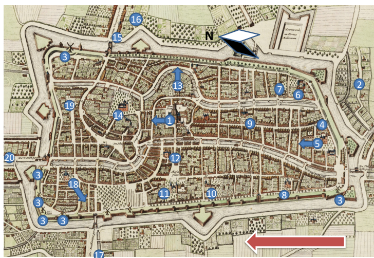
Figure 5. Compiled damages to larger structure in the city of Utrecht. The number is in blue circles refer to table 1, the blue arrows refer to the direction in which the structure collapsed (details in sect. 3.2). The large red arrow denotes the direction in which the front moved over Utrecht. Map from J. Bleau (1649), Utrecht City Archive no. 214022.
