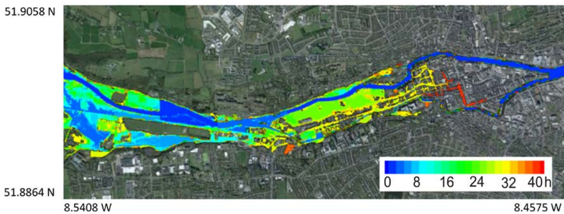
961 Figure 16: Maps of flood inundation observed by (a) OPW and (b) modelled (contours represent 2-hour 962 intervals). Evolution of modelled flood wave is a combined output of CG06 and CG02 models.
