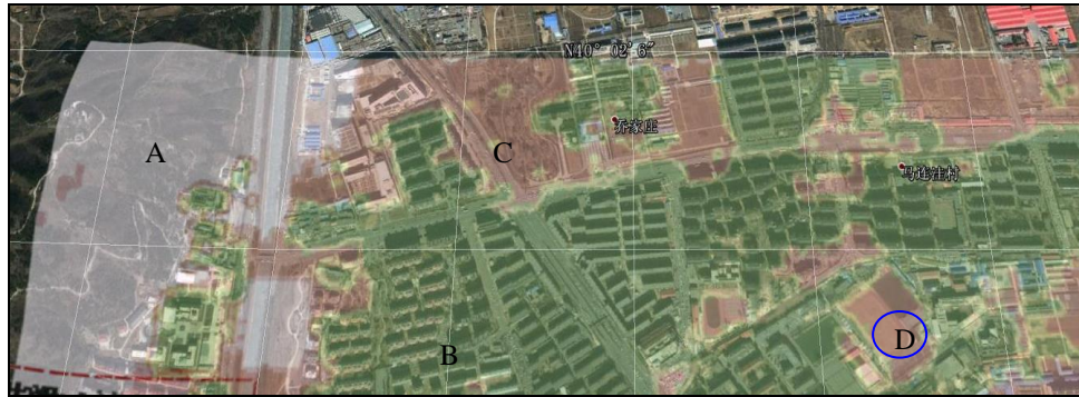
Figure 4-5 Sensitivity zones in the sub-district of Malianwa, in case of (a) not accounting for the terrain factor, (b) accounting for terrain factors, (c) and displayed in Google Earth; these zones correspond well with the distribution of underlying structures and topographical features. For example, point A in the mountainous areas exhibits a high sensitivity, B in the dense structure areas exhibits a lower sensitivity on account of lightning rod effects produced by nearby structures, and C in an open-field area exhibits a relatively high sensitivity. Interestingly, the sensitivity of point D at an open sports field is obviously higher than that of its surrounding densely built-up areas.
