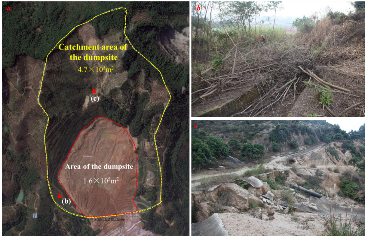
Fig. 5 a An overview of the catchment area (Google Earth image); b The surrounding peripheral drainage channel of the dumpsite was abandoned; c Damaged drainage pipes were not repaired and failed to divert surface run-off into the peripheral drainage channel. Surface run-off concentrated in the waste filling.
