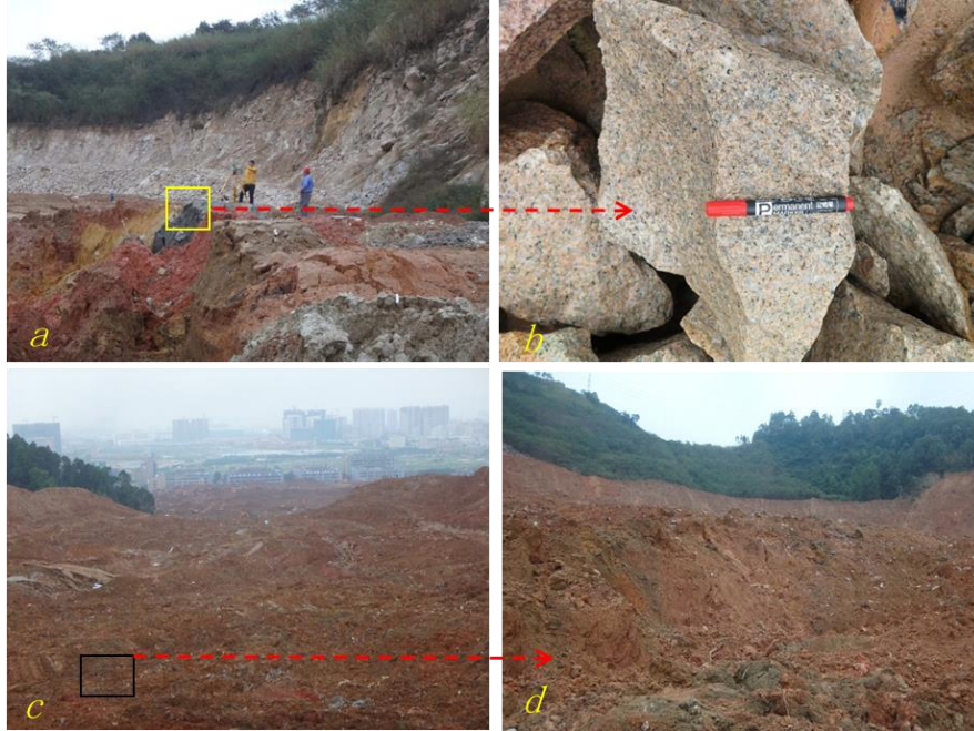
113 Fig. 2 Photos of the rock and soil specimen collected from the displaced material. a Exposed granite rock 114 near the flowslide scarp; b Close view of the granite rocks; c Displaced material in the zone of depletion; 115 d Materials in the flowslide source area.
