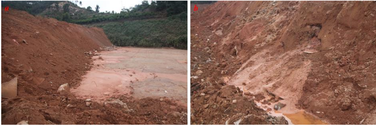
Fig. 16 Evidences of liquefaction near the opening of the failed slope.
