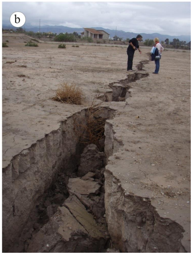
570 Figure 12. Compaction on clay soils interpreted as due to compressibility after groundwater overexploitation. A. Large crack development on vertisols on Béjar fan distal area (Source: La Verdad de Murcia). B. Crack detail up to 150 cm width and 2 m height.
