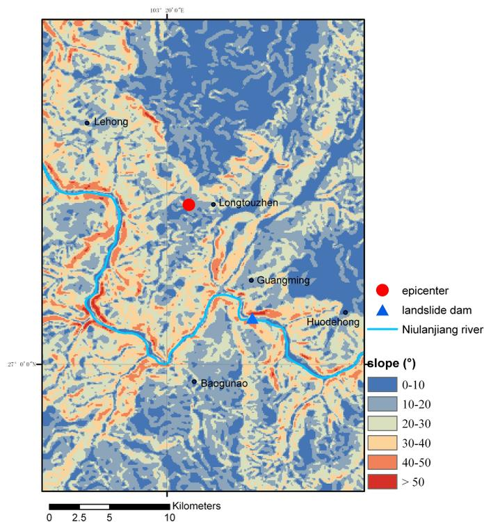
**Fig. 1.** Figure 3. Map showing slope angles in the Ludian seismic area
