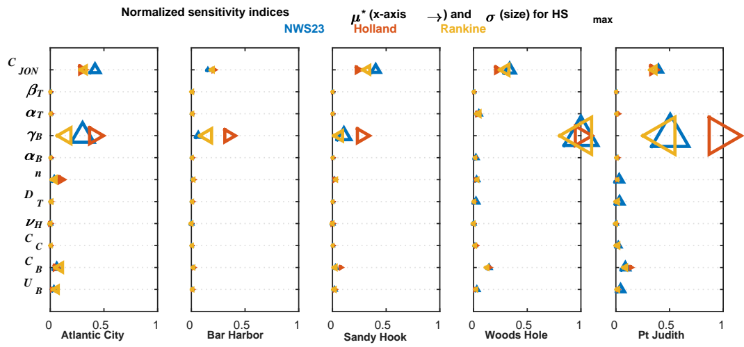
Figure 5. Campolongo sensitivity indices for wave height at buoy locations for different wind models: blue upward pointed triangle – NWS23, brick right pointed triangle – Holland, mustard left pointed triangle – Rankine. Triangle size proportional to \sigma index.
