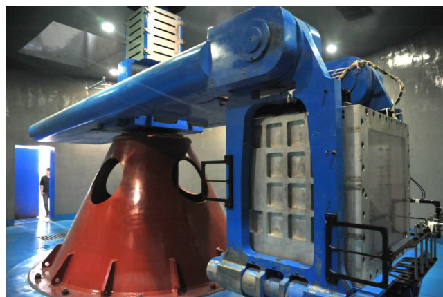
Figure 26. The geotechnical centrifuge used in experimental modeling.
