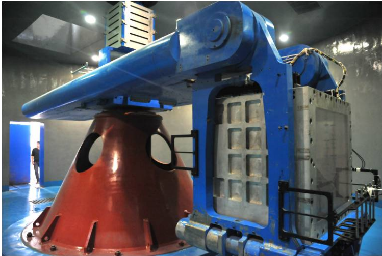
Figure 26. The geotechnical centrifuge used in experimental modeling.
