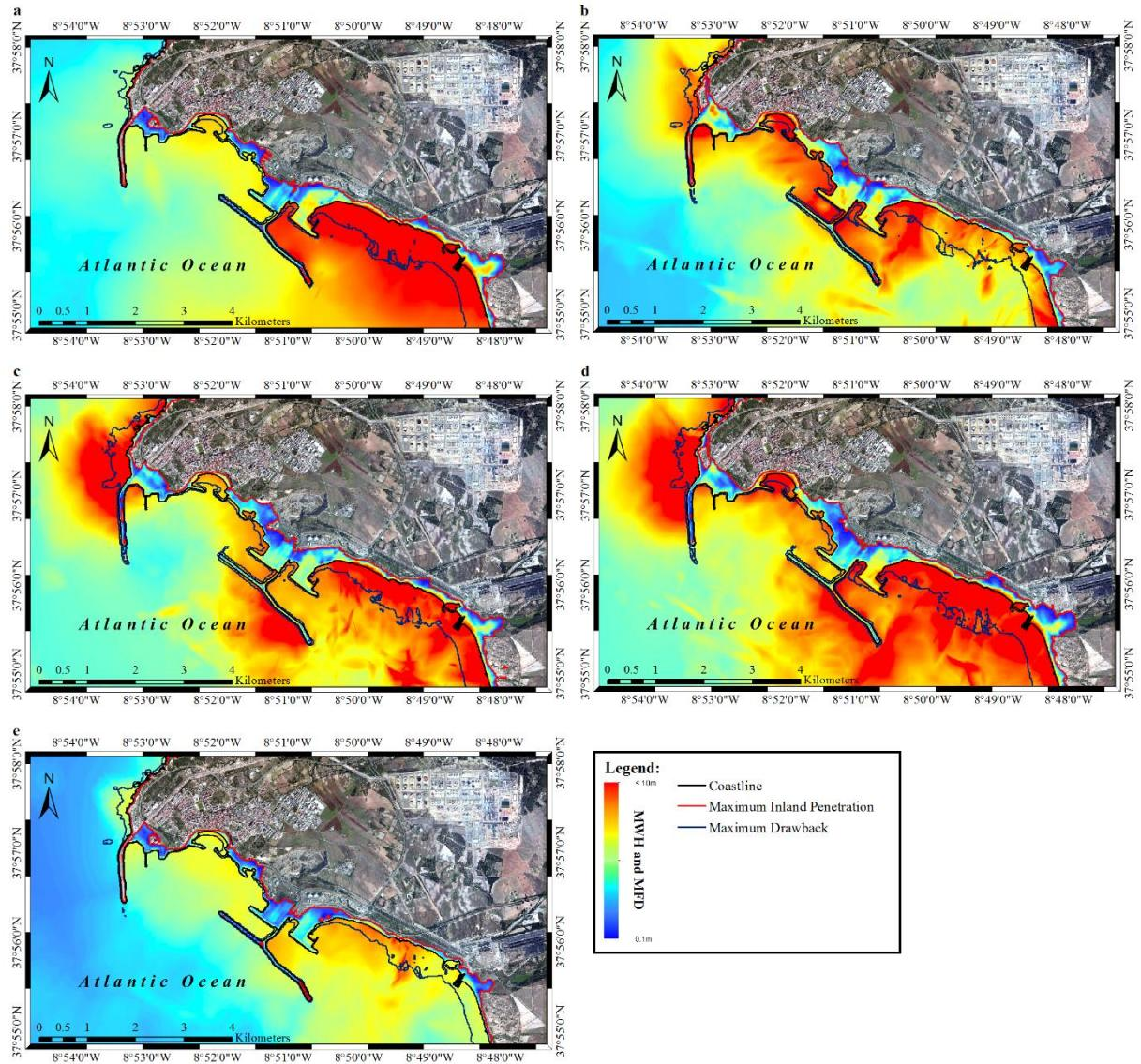
Figure 3. Results of MWH, MFD, MDB, MIA and MIP of the SWIM scenarios considering MSL: (a) CWF, (b) GBF, (c) HSF, (d) HSMPF, (e) MPF. MWH and MFD are presented by the colour bar in the lower right corner offshore and on land respectively. Offshore and land are separated by the coastline (black line). MDB is indicated by the dark blue line. The MIA is given between the coastline and the MIP (red line).
