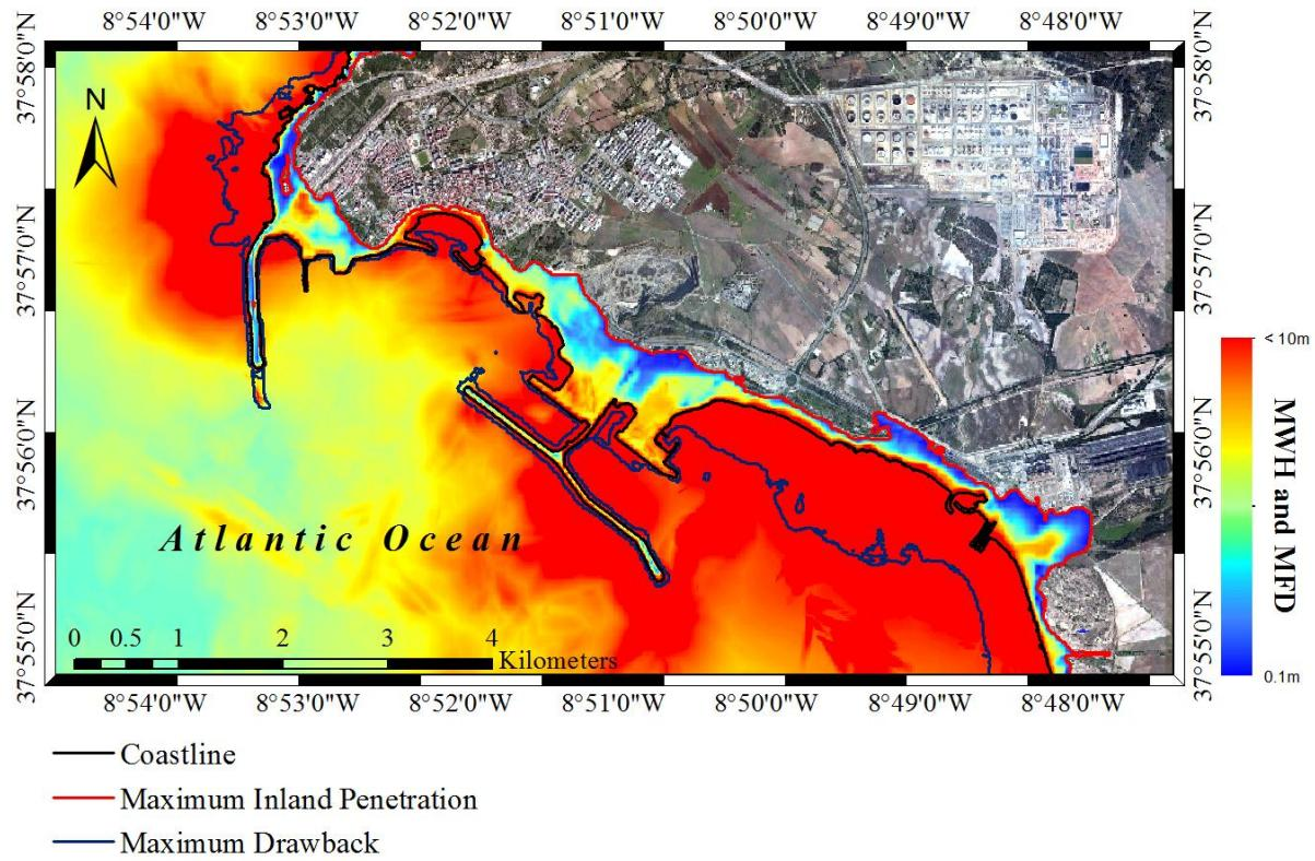
Figure 6. MWH, MFD, MDB, MIA and MIP for the aggregate scenario considering all stages of the tide. MWH offshore and MFD on land are presented by the colour bar. MDB is indicated by the thick dark blue line. The MIA is given between the coastline (black line) and the MIP (red line).
