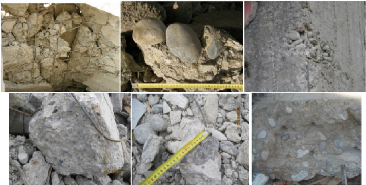
Figure 28. Concrete and aggregate samples in a single-story reinforced concrete building that collapsed in the Van Organized Industrial Site [20], and a concrete cross-section displayed in the wreckage [17].
