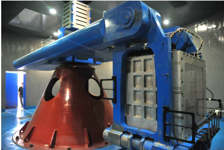
Figure 26. The geotechnical centrifuge used in experimental modeling.
