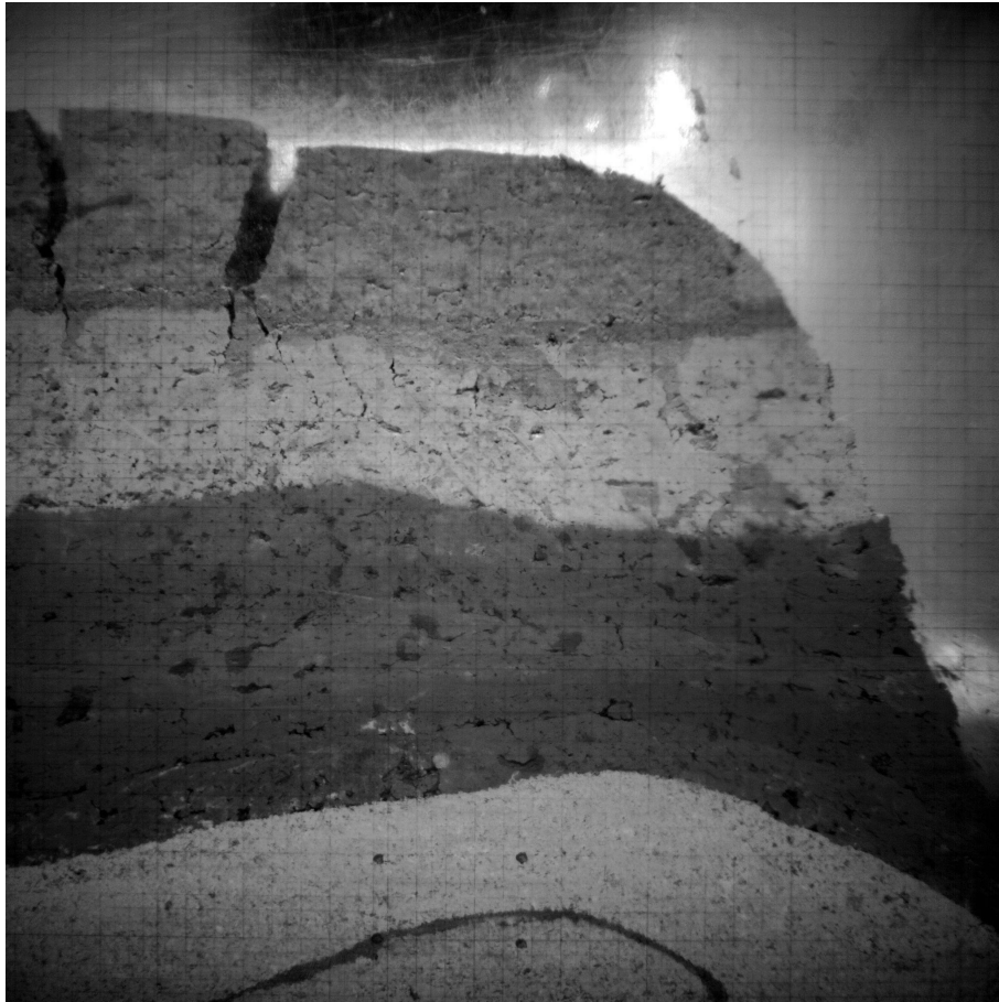
Figure 30. Going cracking and shear creeping at the bottom.
