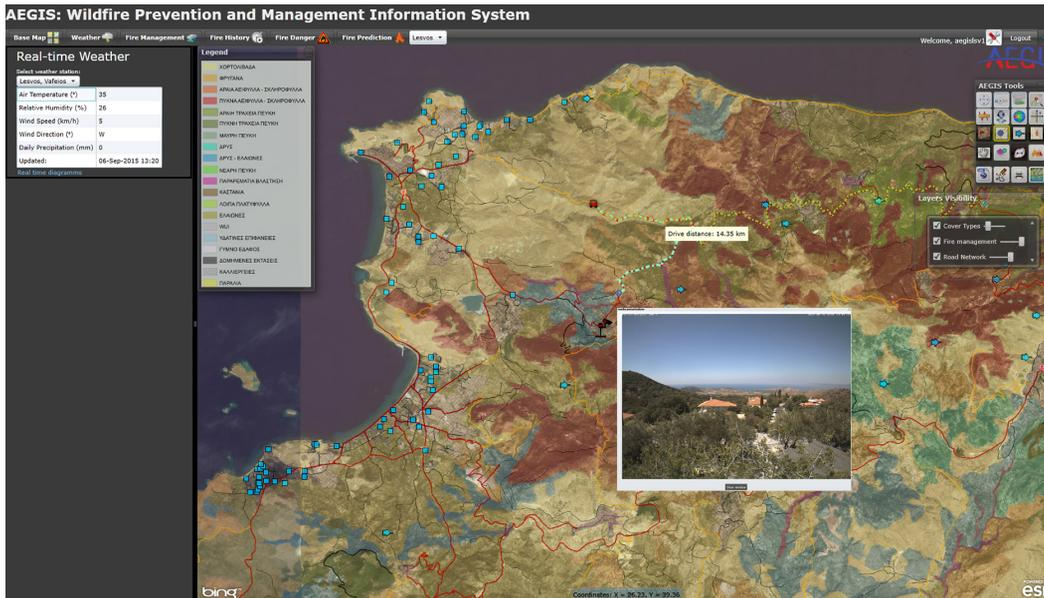
**Figure 6.** Optical camera surveillance combined with visualization of the road network, the pumping stations, the cover types and real-time weather records from the closest RAWs within the AEGIS graphical interface.
