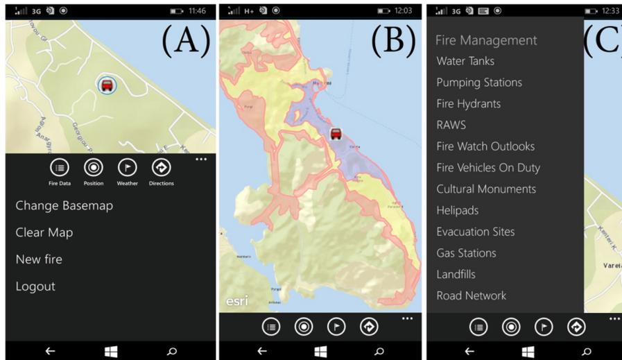
**Figure 8.** (a) Basic screen of AEGIS App; (b) calculation of the areas that the user can access by driving a regular firefighting truck in 3, 5 and 10 min; and (c) accessing fire management data through the AEGIS App.
