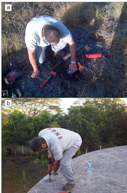
Figure 7. Installation of (a) Lacayo benchmark on rocky lava outcrop and (b) Tanque benchmark on existing reinforced concrete structure.
