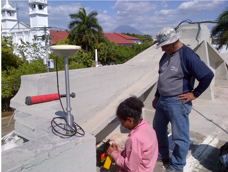
Figure 9. Close-up of the self-centering mount at the Usulután site and training of the MARN personnel in the field.
