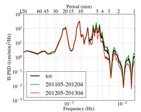
**Figure 5.** Average power spectra of the sea-level slope function IS computed with  $T_{IS} = 4$  min. For further details see caption of Fig. 3.
