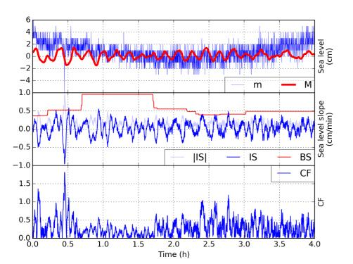
Figure 1. Sea-level of the Siracusa tide-gauge (top panel), the corresponding sea-level slope IS and background slope BS (second panel), the filtered sea-level SL and the control function CF for a sample of 4 h.
