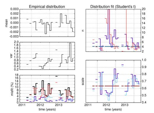
**Figure 13.** Statistical analysis of SL. See captions of Fig. 12 for details. The measure units are cm for the mean and for the scale parameter S, and cm<sup>2</sup> for the variance. The long-term estimates for n and S are respectively 4.25 and 0.64 cm.
