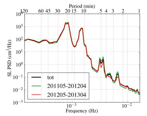
**Figure 6.** Power spectra of the long-wave sea-level function SL, computed with  $T_{IS} = 4$  min and  $T_{SL} = 10$  min. For further details see caption of Fig. 3.
