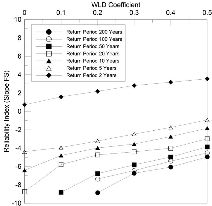
**Figure 12.** Variations in the slope FS reliability index with the WLD coefficient for various flood return periods, with accounting for the variability of the in-situ friction angle.
