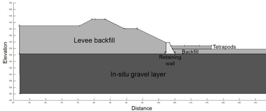
**Figure 2.** Simplified cross-section of Chiuliao 1st Levee before Typhoon Morakot (modified from Huang et al., 2014).
