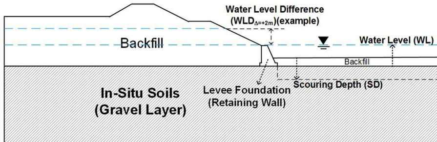
**Figure 4.** Definitions of the parameters (WLD, WL, and SD) used in levee stability analyses (Huang et al., 2014).
