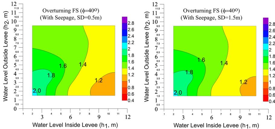
**Figure 7.** Retaining wall overturning safety factor of Chiuliao 1st Levee for SDs of 0.5 m (left panel) and 1.5 m (right panel).
