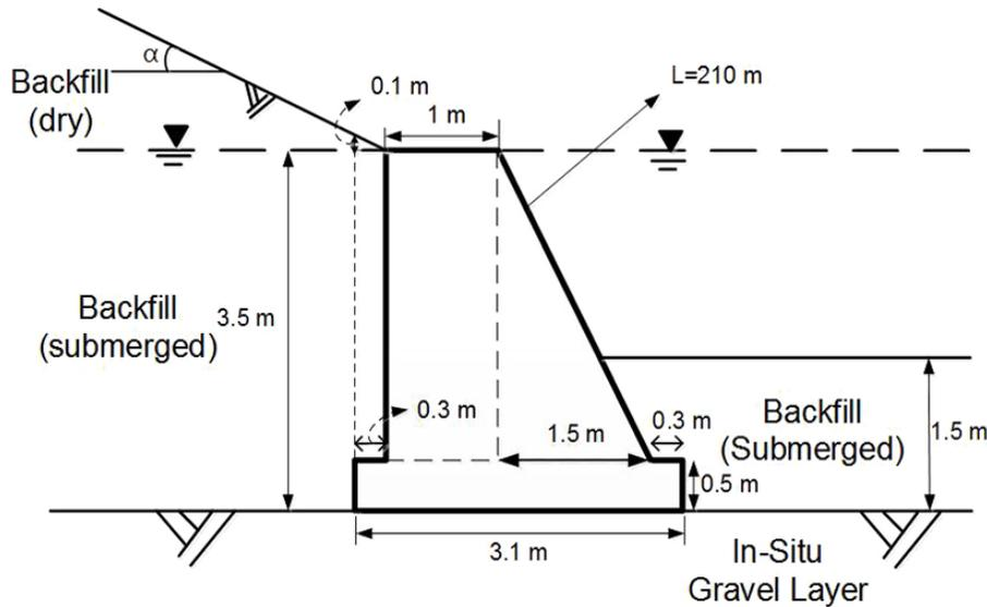
**Figure 3.** Cross-section of the retaining wall of Chiuliao 1st Levee (Huang et al., 2014).
