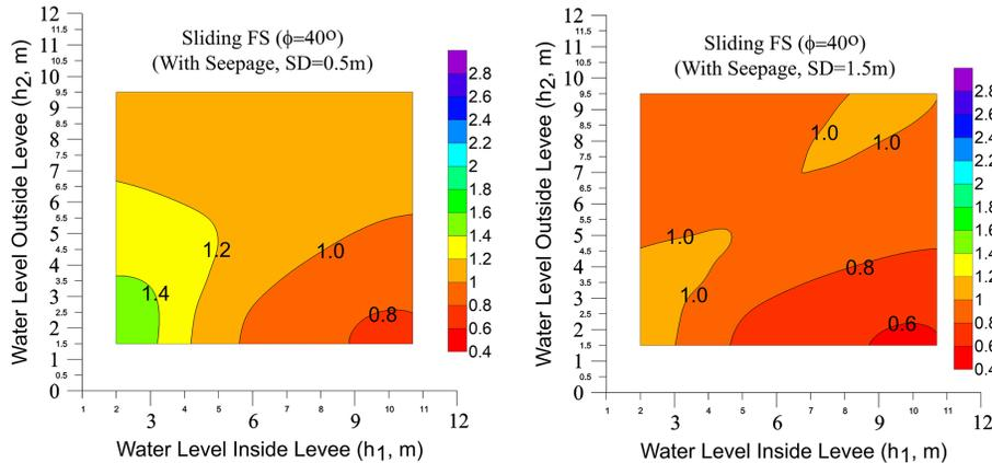
**Figure 6.** Retaining wall sliding safety factor of Chiuliao 1st Levee for SDs of 0.5 m (left panel) and 1.5 m (right panel).
