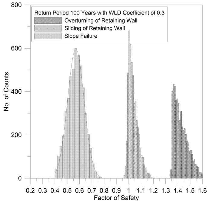
**Figure 11.** Distributions of the safety factor for various failure mechanisms, with accounting for the variability of the in-situ friction angle (results shown here are for a flood return period of 100 years and a WLD coefficient of 0.3).
