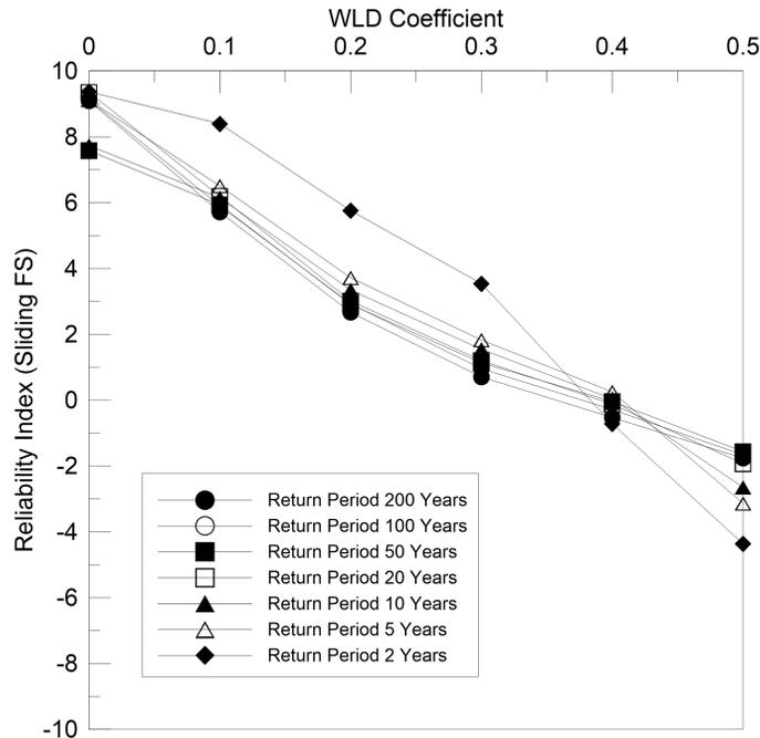
**Figure 13.** Variations in the retaining wall sliding FS reliability index with the WLD coefficient for various flood return periods, with accounting for the variability of the in-situ friction angle.
