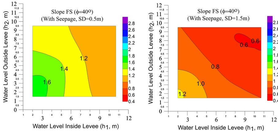
**Figure 5.** Slope stability of Chiuliao 1st Levee for SDs of 0.5m (left panel) and 1.5 m (right panel).
