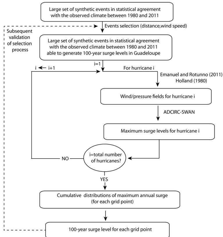
**Figure 3.** Schematic diagram of the method used to estimate 100 year surge levels. The same approach is followed for the 1000 year return period, but with a larger set of synthetic storms and different criteria to select the events to be computed.
