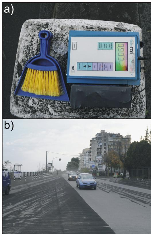
**Figure 2.**  $PM_{10}$  measurement carried out on 15 November 2011 in Acireale at site 2 (SS114 road): **(a)** DustTrak working; the display shows the averaged reading over the previous 10 s; **(b)** transit of cars at the crossing.
