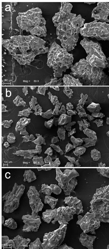
**Figure 6.** Scanning electron microscope secondary electrons (SEM-SE) images representative of the textures identified in studied tephra showing moderately vesicular, glassy scoriaceous fragments with fluidal texture (sideromelane) and scarce poorly vesicular, blocky clasts (tachylite). **(a and b)** PM<sub>1</sub> sample at Fleri; **(c)** PM<sub>2</sub> sample at Acireale.
