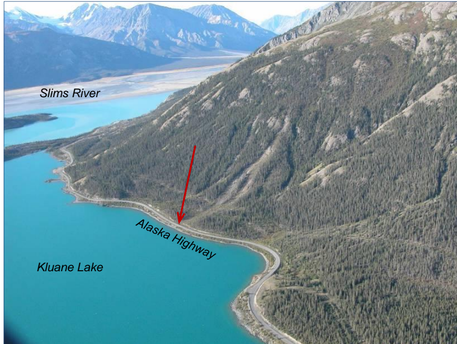
Figure 9. Oblique photo of debris flow channels at Horseshoe Bay, southwestern end of Kluane Lake (photo by C. Huscroft). During the 1988 storm event, debris flow deposits blocked the Alaska Highway (e.g., red arrow) for up to seven days (Evans and Clague, 1989). Site F in Figs. 7 and 8b).
