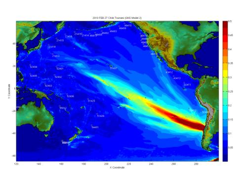
**Figure 1.** The maximum wave height from the Chile 2010 tsunami calculated with the COMCOT model. Also shown are the locations of the DART gauges at the time of the event. From Power (2013).
