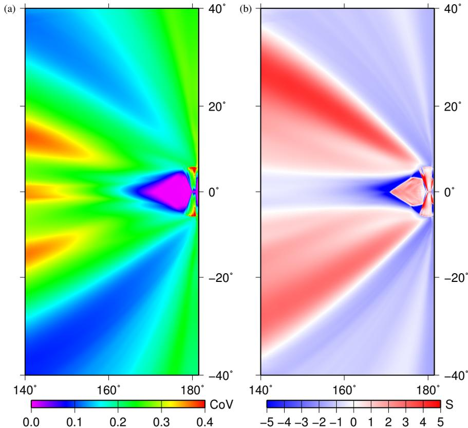
**Figure 10.** The effect of having a step in the bathymetry on the CoV and skewness of  $h_{\max}$ . **(a)** shows the CoV from a set of  $M_w$  9.5 events with a  $\sigma_{\text{strike}} = 10^\circ$ . The elevation has a step at  $182.5^\circ$  where it suddenly increases to 100 m above mean seal level. The other parameters are otherwise the same as in Fig. 4b. **(b)** The effect of the step on the skewness of the distribution of the maximum tsunami wave heights (cf. Fig. 5b).
