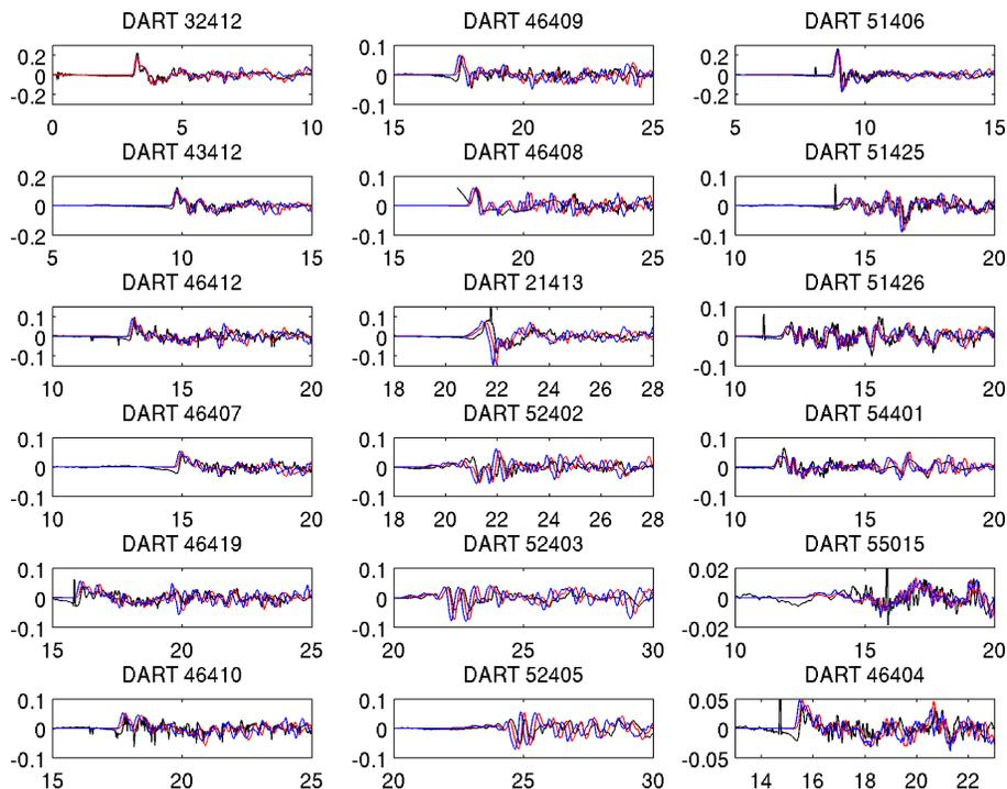
**Figure 2.** The de-tided mareograms at selected DART stations from the 2010 Chile tsunami (black). Also shown are the tsunami waveforms calculated using the COMCOT (red) and the EasyWave models (blue) from a simplified source model for this event. The y axis shows the wave height relative to mean sea level in m, while the x axis shows the number of hours after the earthquake occurred.
