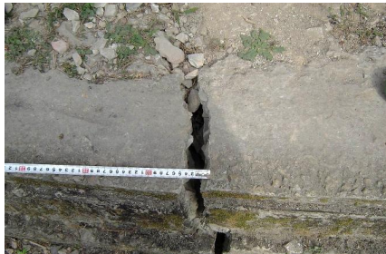
Figure 6. Photo of cracks in farmland at elevation 692 m.
