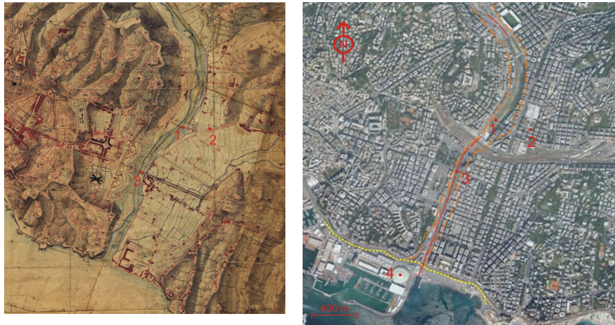
Figure 6. Final stretch of the Bisagno Stream at the beginning of the 19th century (left) and to present day (right). Note the complete urbanization, the progradation to the sea in the Piazzale Kennedy area and Fiera del Mare (4) and the narrowing of the flow section near the S. Agata bridge (1) and of Pila bridge (S. Zita) (3). Number 2 shows the Sant'Agata Cloister, where the left shoulder of the bridge rose (280 m length). Note that the stream is completely culverted downstream the railway since “30”s (red dashed line). In orange dashed line we can see the Bisagno Stream banks at the beginning of 1800; in yellow dashed line the shoreline at the beginning of 19th century.
