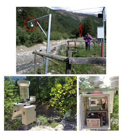
**Figure 2. (a)** The most upstream of the fixed video cameras (red circle) of the Gadria instrumented area, which is part of the EWS testing field installation, the arrow indicates the position of the flashing light; **(b)** the ALMOND-F equipment allowing the implementation of different types of warning algorithms; **(c)** detail of the equipment.
