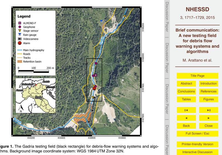
Figure 1. The Gadria testing field (black rectangle) for debris-flow warning systems and algorithms. Background image coordinate system: WGS 1984 UTM Zone 32N.
