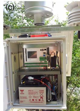
**Figure 2.** (a) The most upstream of the fixed video cameras (red circle) of the Gadria instrumented area, which is part of the EWS testing field installation, the arrow indicates the position of the flashing light; (b) the ALMOND-F equipment allowing the implementation of different types of warning algorithms; (c) detail of the equipment.
