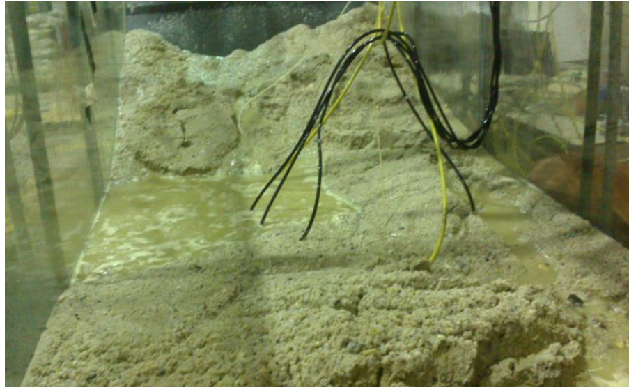
Figure 14. Slope failure (flowslide).
