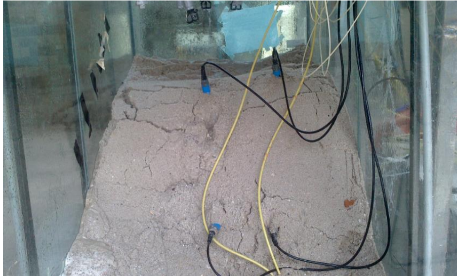
Figure 17. Slope failure (flowslide).
