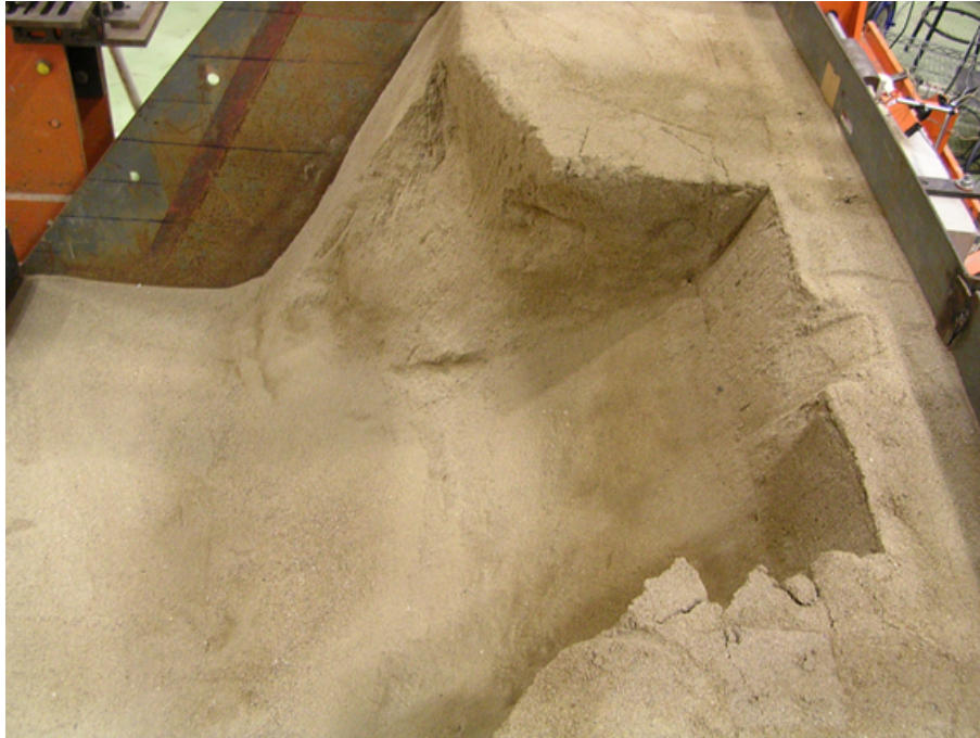
Figure 10. Global three-dimensional slope failure.
