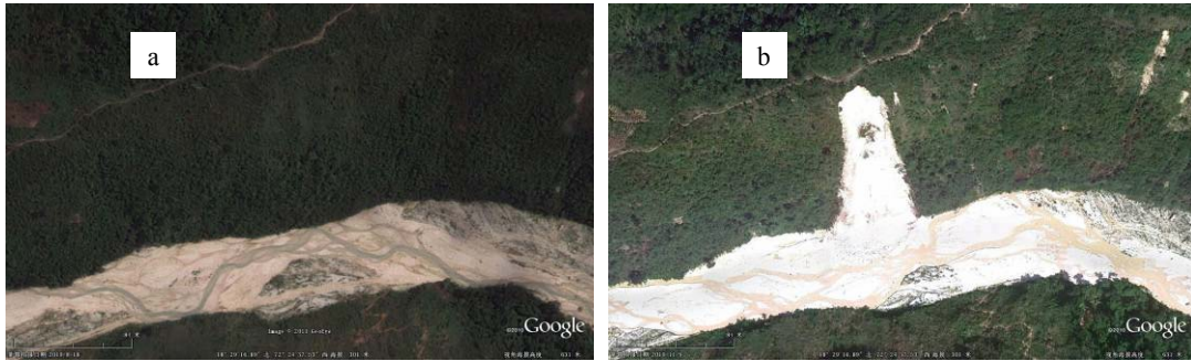
Fig. 4 A landslide ( 18^{\circ}29'16.89''\text{N} , 72^{\circ}24'37.53''\text{W} ) occurred after the earthquake but may be triggered by rainfall. a was taken on 18 August 2010 and b was taken on 9 November 2010.
