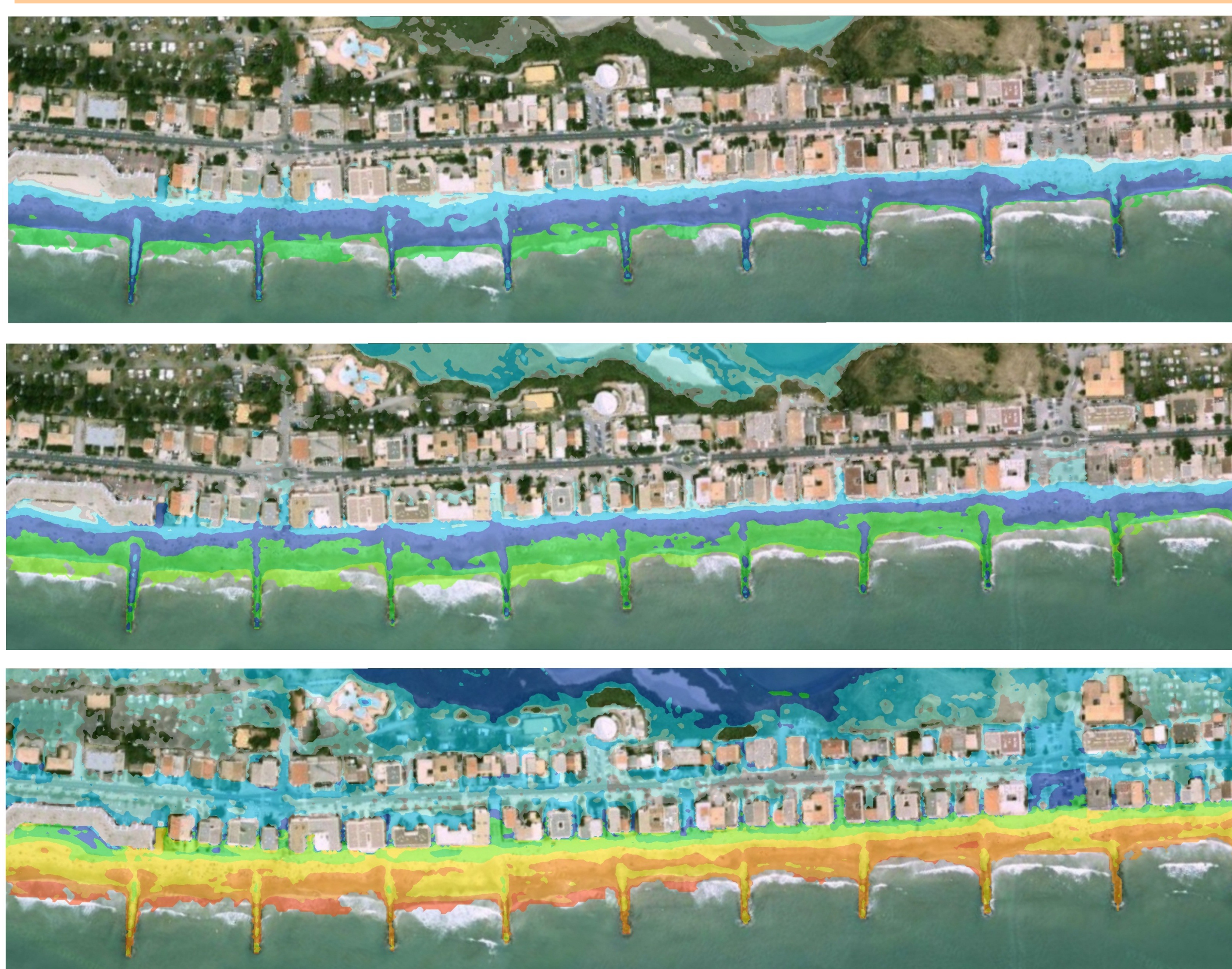
Maximal water height (m) in the inundation area : top, at the present ; middle with a 0.35m of sea level rise ; bottom with 1m of sea level rise.
