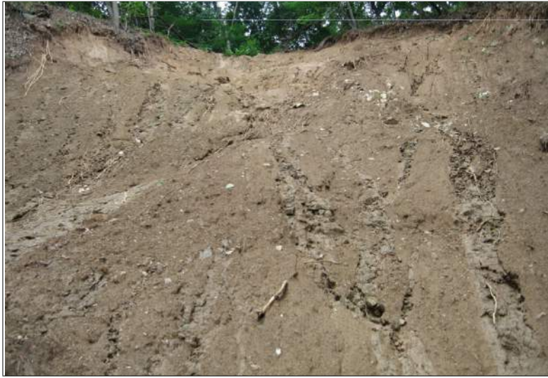
Figure 5a. Landslides in Site B. a. A closer look of the landslide Initiation zone. A small volume of soil slid down along the smooth clayey surface which acts as a slickensided shear plane. b. Upstream valley where debris flows were traced. Looking northwest.
