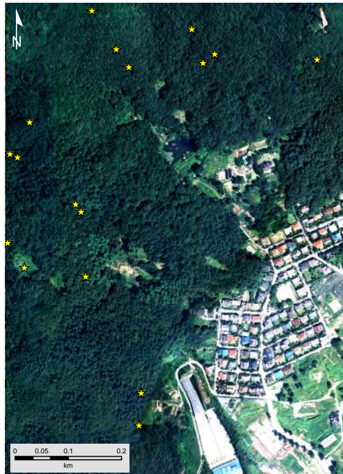
Figure 12a. Landslides characteristics in Site B. a. Aerial photograph, before the landslide. Yellow stars represent landslide initiation zones. b. Modified Planarity. Areas outlined by yellow circles with a diameter of 5 m are supposed to the source areas. c. Aerial photograph, after the landslide. Orange lines indicate observed routes from the landslide initiation zones.
