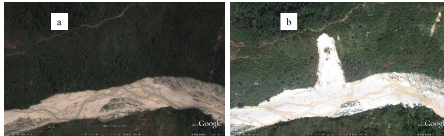
Fig. 4. A landslide ( 18^{\circ}29'16.89'' N, 72^{\circ}24'37.53'' W) occurred after the earthquake but may be triggered by rainfall. (a) was taken on 18 August 2010 and (b) was taken on 9 November 2010. Upward is north.
