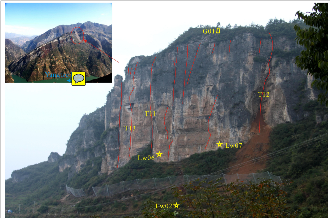
Fig. 11 Overview of Wangxia Cliff prior to the catastrophic rock slump. G01 represents a GPS station, and Lw02–Lw07 indicate the displacement monitoring stations. The rock slump of October 21, 2010 was controlled by vertical scars T11 and T12. The red lines represent fissures in the rock mass.
