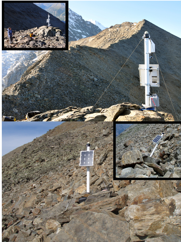
Fig. 1. GPS stations of pos27 (top) and pos55 (bottom). The small photo (bottom right) shows GPS station pos55 at the end of June 2012, by then the station is strongly tilted towards the slope. Each GPS station includes a GPS antenna and two inclinometers that are mounted on top of a mast. The energy to operate the devices is provided by a photovoltaic energy harvesting system and backed by a battery. (Photos: V. Wirz and R. Delaloye)
