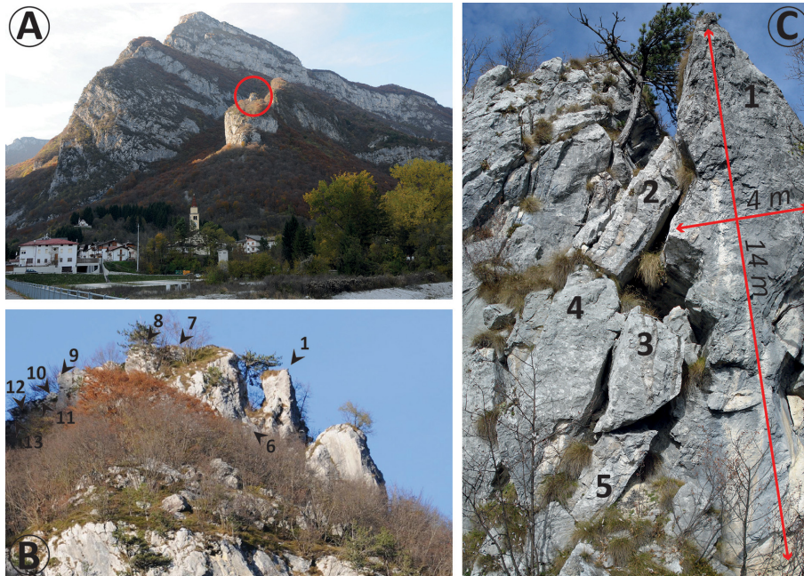
Figure 2. Panoramic view of Cimolais Village and overlying Crep Savath peak (a). The red circle indicates the rock fall source areas. The oblique view from Fesena Valley (b) and the frontal view (c) highlight the hazardous position and the large dimensions of Block 1.
